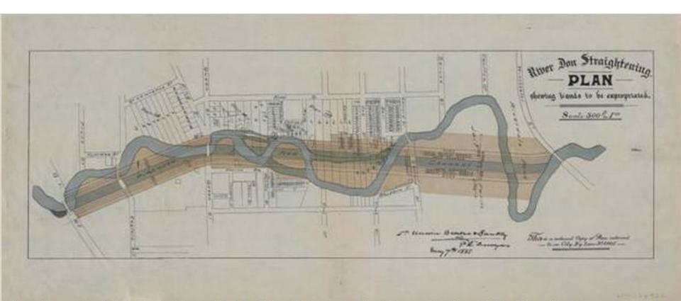
River Don Straightening Plan, 1886, City of Toronto Archives, Series 725, File 12. Concentrating on a portion of the Lower River between Winchester Street and the Grand Trunk Railway bridge at Eastern Avenue, the Don Improvement Plan (1886-1891) saw the meandering Lower River straightened, widened, and deepened, dramatically transforming the landscape and hydrology of the marshy lower valley.
